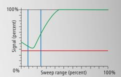
The CleverLevel LFFS switch is the solution: Thanks to its frequency sweep technology and its ability to analyze the strength of the signal, and the signal dumping which differs from media to media. The switch can be set to trigger only on the specific medium even if both media involved have the same Dk value.
